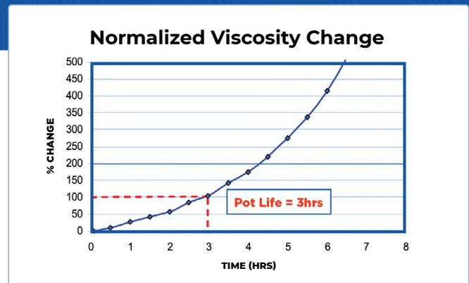
Pot life, working life, and gel time are properties of an epoxy that can vary greatly from product to product. These properties play a vital role in material selection when choosing an adhesive for a specific manufacturing environment or process. When selecting an epoxy, pot life may be an important concern for one application, but not for another. When it matters, it is important to know how to interpret product test data on a product's datasheet concerning these properties.
